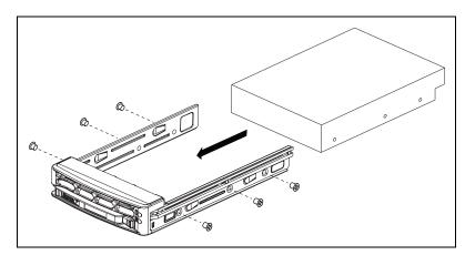
Figure B-27. Sliding Hard Disk Drive into SCA Drive Tray
